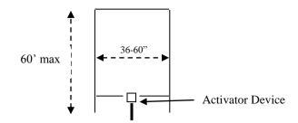
To install the activator loop, cut a groove approximately ¼ inch (6-8 mm) wide and ½ inch (12-13 mm) deep in the track with the dimensions shown below. For dirt tracks, place the activator loops in plastic PVC sprinkler pipes. Make sure the pipes are sealed such that water will not enter the pipes. Once the loop has been created and installed, the banana plugs at the ends of the loop should be inserted into the loop inputs on the activator device.
