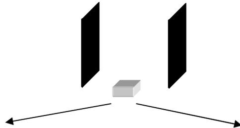
**Good location:** No metal to block the signal. The detection window is very wide.
