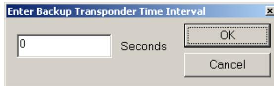
If the primary transponder is not detected either due to malfunction or has fallen off the vehicle, the backup transponder will be used. However, Race Manager will always display the primary transponder number.
